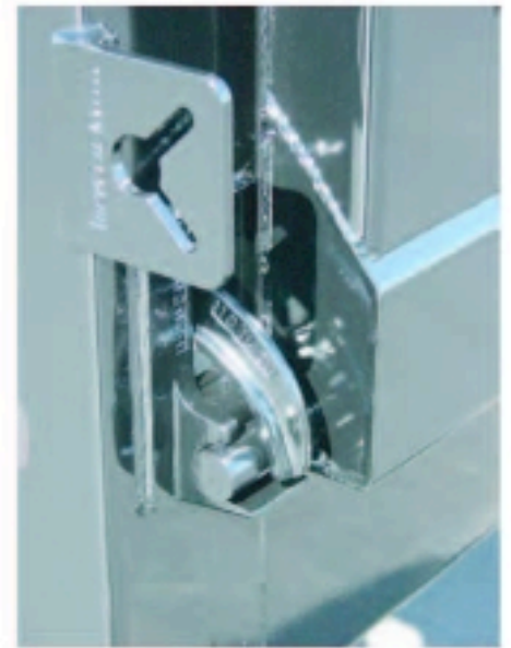
Lower tailgate latch is 4140 grade cast steel. Latch pivots are bushing type width 1 1/4" diameter pin for extra support.
