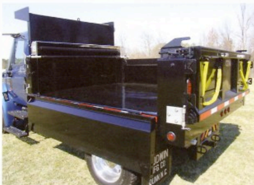
Shown is one of the sides in the down position. The side easily unlatches with a single handle and folds down lower than the body floor for greater access to the interior.
