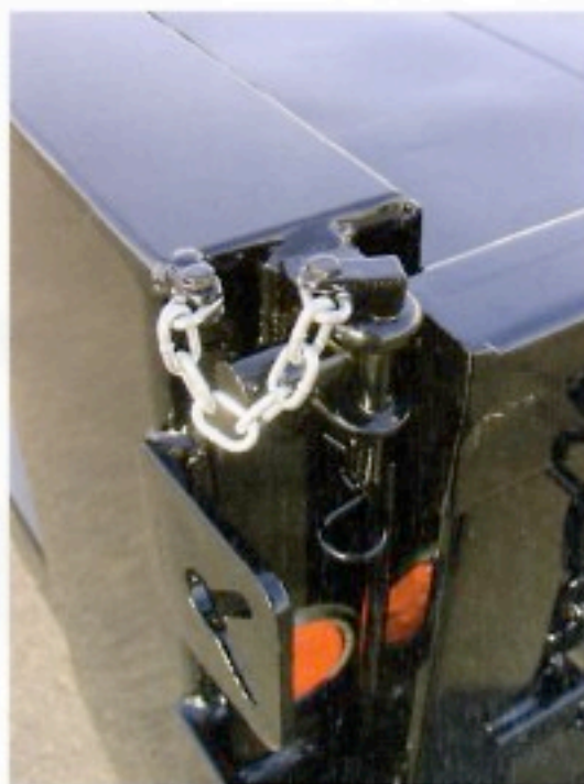
Shown is the standard F-latch upper hardware with keeper chain.
